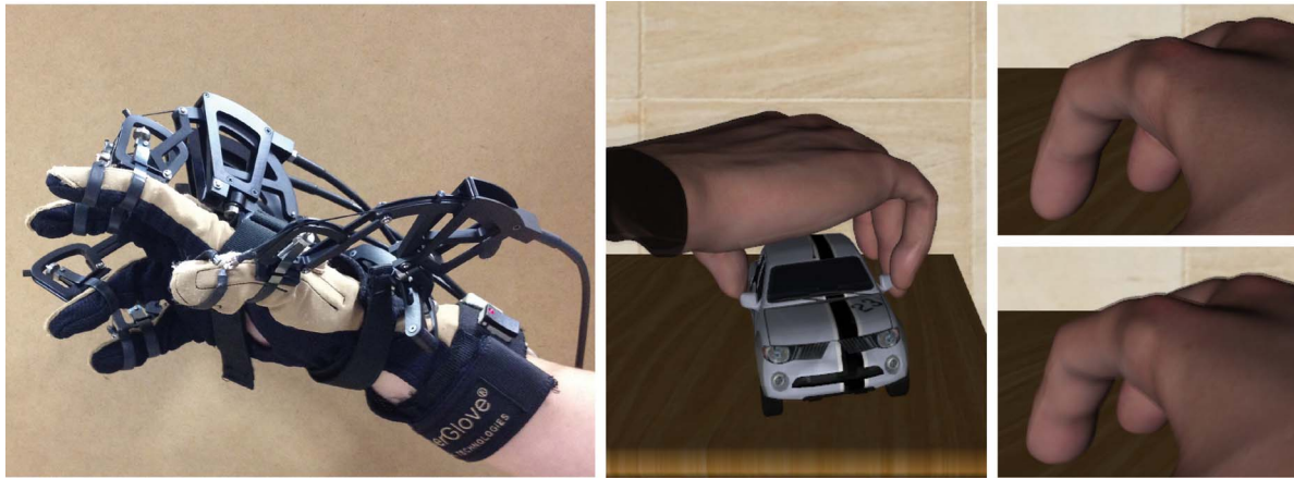
Fig. 6. (Left) Cybergrasp exoskeleton device with hand tracking and tactile feedback on the fingertips. (Middle) Interactive hand simulation for haptic rendering of grasping and manipulation tasks [57]. (Right) Detailed fingertip deformations that require combined kinesthetic and cutaneous haptic rendering.
