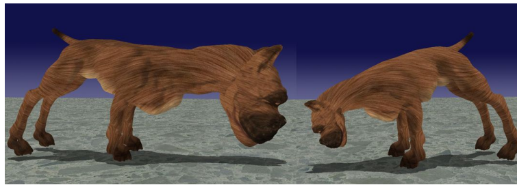
Figure 4.3: The pitbull with its inflated head (left) shows the artifact of linear FEM under large rotational deformations. The correct deformation is shown on the right.
