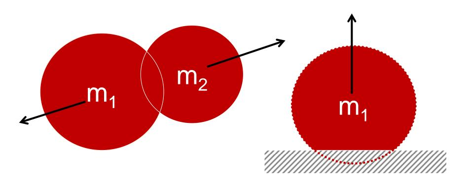
Reaction forces are computed between mass nodes
